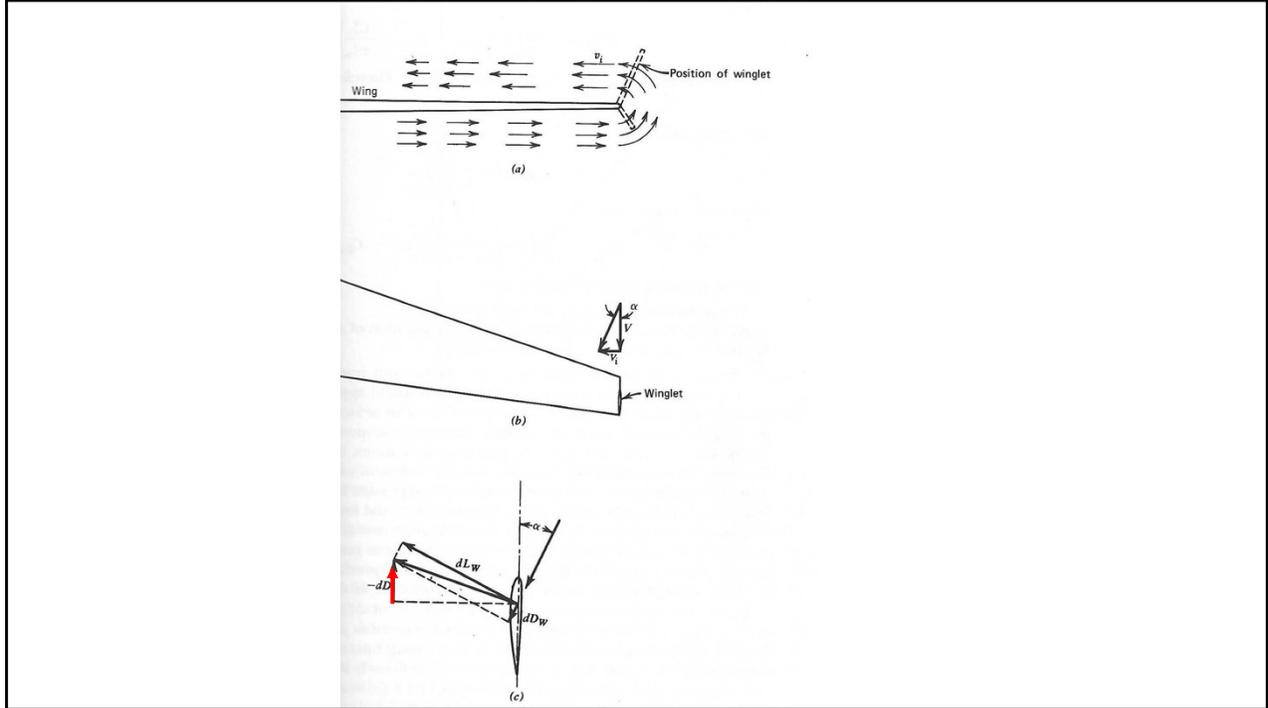
The main goal of winglets is to reduce induced drag. Only a detailed flow analysis can provide exact gains, but the following qualitative analysis gives an indication on how a gain is possible.
