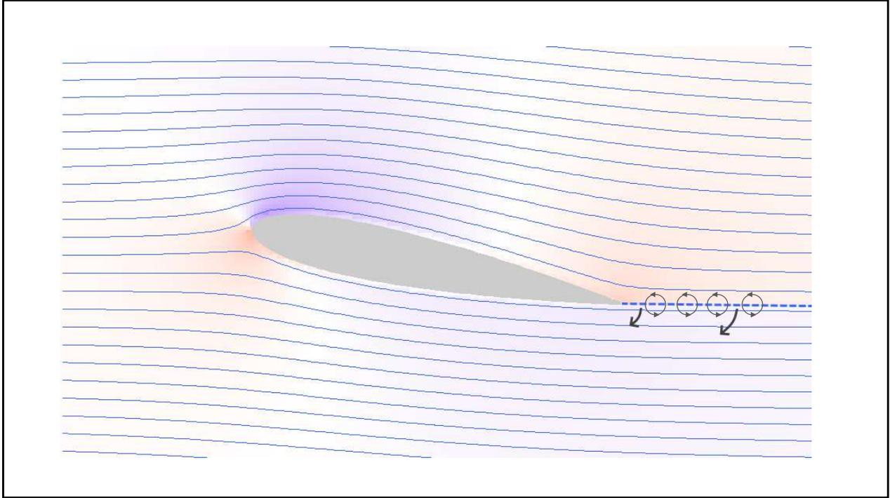
First, let's note that the previously mentioned shear layer that develops upon starting the flow can be also be viewed as a vortex sheet—see rationale on slide no. 6.
