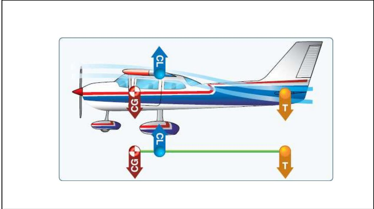
The traditional way to stabilize the system is to move the CG ahead of the center of lift of the wing, and add a stabilizer surface downstream of the wing, with a downward lift. As a result, the wing will have to provide additional lift (weight + T, vs. weight only).
