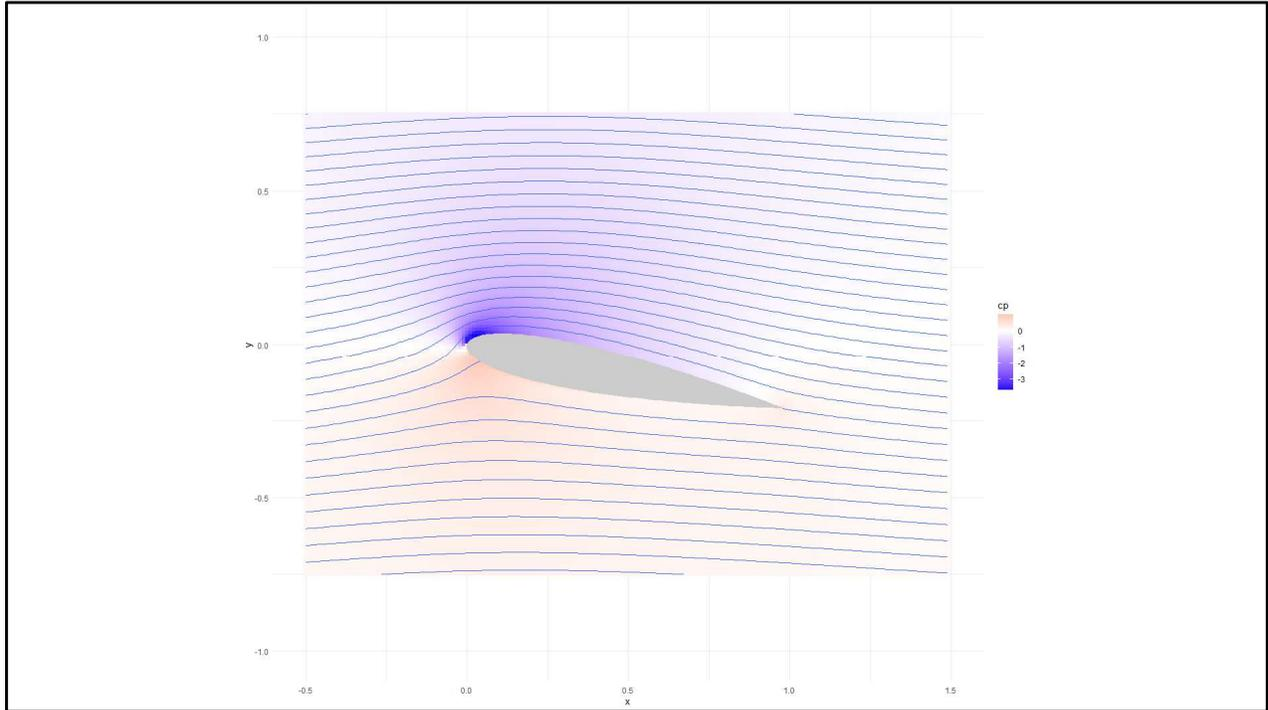
Lift arises from the difference in pressure between the top of the airfoil (where the pressure is less than ambient) and the bottom (where the pressure is higher than ambient).
