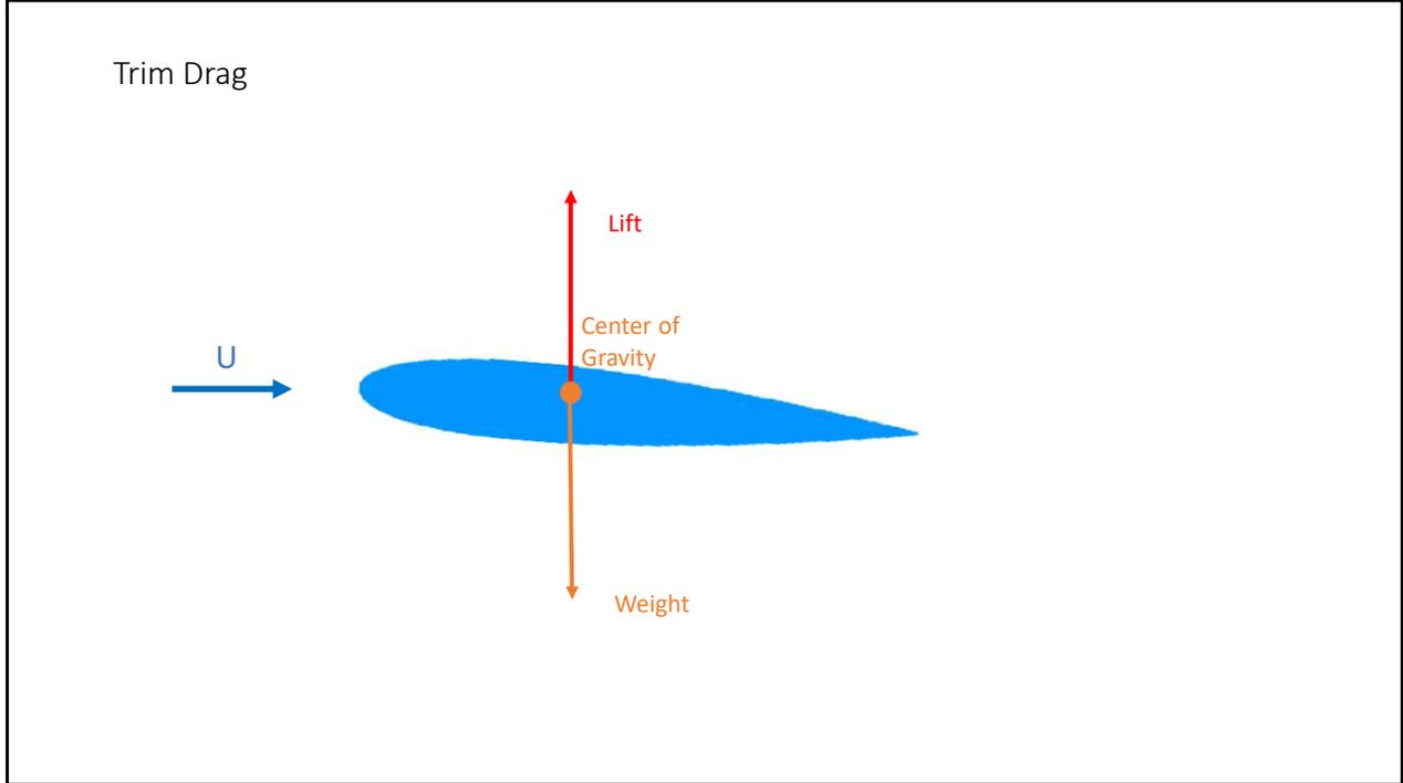
Consider a single wing in straight-and-level flight. The weight acts through the center of gravity. For the wing to be in equilibrium, the lift vector must also be applied to the center of gravity.
