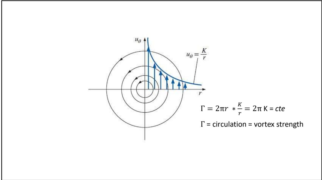
And here is a representation of a single vortex. The flow rotates around the axis of a circular cylinder, with a speed inversely proportional to the radius—we can imagine it as a small tornado!
