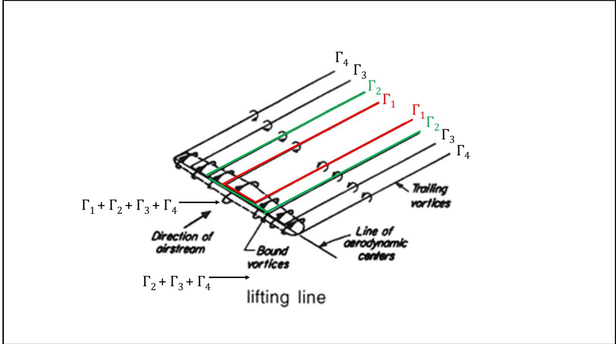
Now, the horseshoe vortex model is an oversimplification. It assumes that lift is constant spanwise until the wingtip is reached—but we just saw that, even in the case of a rectangular wing, the induced velocity will reduce lift. And in the general case of a non-rectangular wing planform, the lift (and thus circulation) will definitely be a function of spanwise location. This can be modeled as nested horseshoe vortices, as illustrated above.
