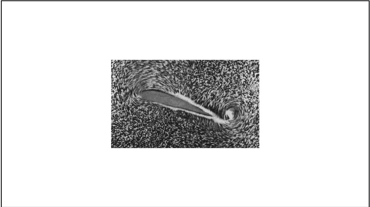
The starting vortex can be observed on the flow visualization above, depicting the flow around an airfoil moments after the flow is started.
