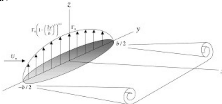
$$D_i = \frac{1}{2} \rho v^2 S C_{Di} \quad C_{Di} = \frac{C_L^2}{\pi A}$$
