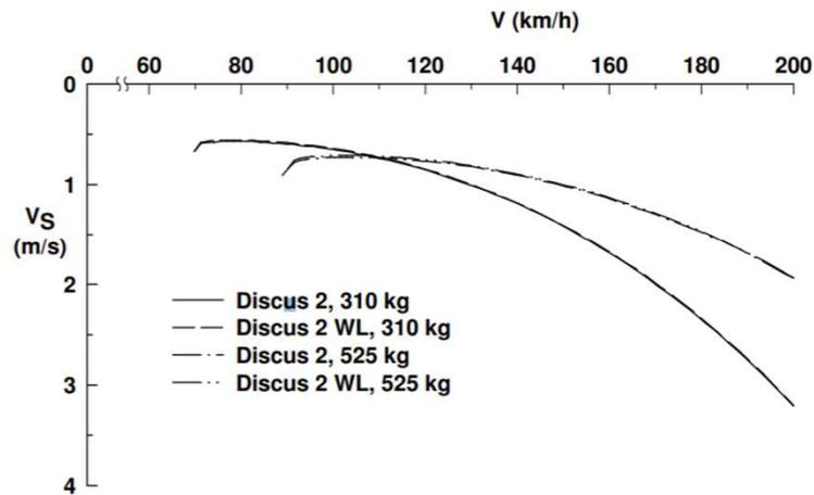
Fig. 8 Predicted straight flight polars of unballasted and ballasted Discus 2, with and without winglets.
