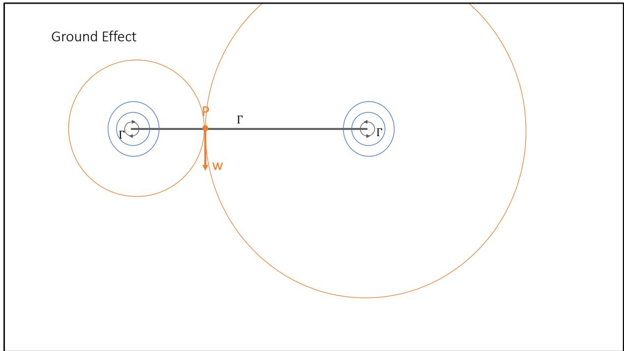
The above diagram illustrates the flow induced by the simplified “horseshoe” model discussed earlier. It presents a view from behind the trailing edge, looking forward. The induced velocity at spanwise location  $P$ , due to the right and left vortices, is represented as the orange vector  $w$ .
