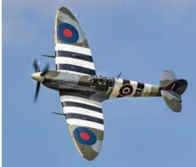
Probably the most famous aircraft using the optimal, elliptically-shaped wing—the Spitfire.
