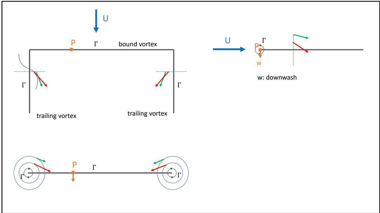
A three-view of the simplified model discussed in the previous slide, with a few selected velocities induced by the trailing vortices. Let's note that the velocity  $\mathbf{w}$  induced at point P, located in the trailing vortices plane at the bound vortex (i.e., at the wing location), is pointing downward.
