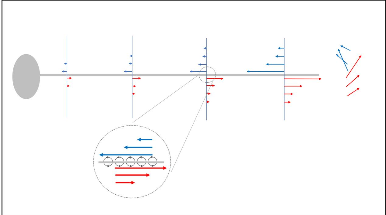
Another way to represent a shear layer is as a “vortex sheet”. We can imagine the shear layer being generated by a large number of tiny vortices leaving the trailing edge in the longitudinal direction (perpendicular to the view above). Considering two adjacent vortices, the vertical velocity components at the trailing edge cancel each other, leaving only the horizontal components. The horizontal velocity is higher closer to the vortex axis and diminishes rapidly with increasing distance.
