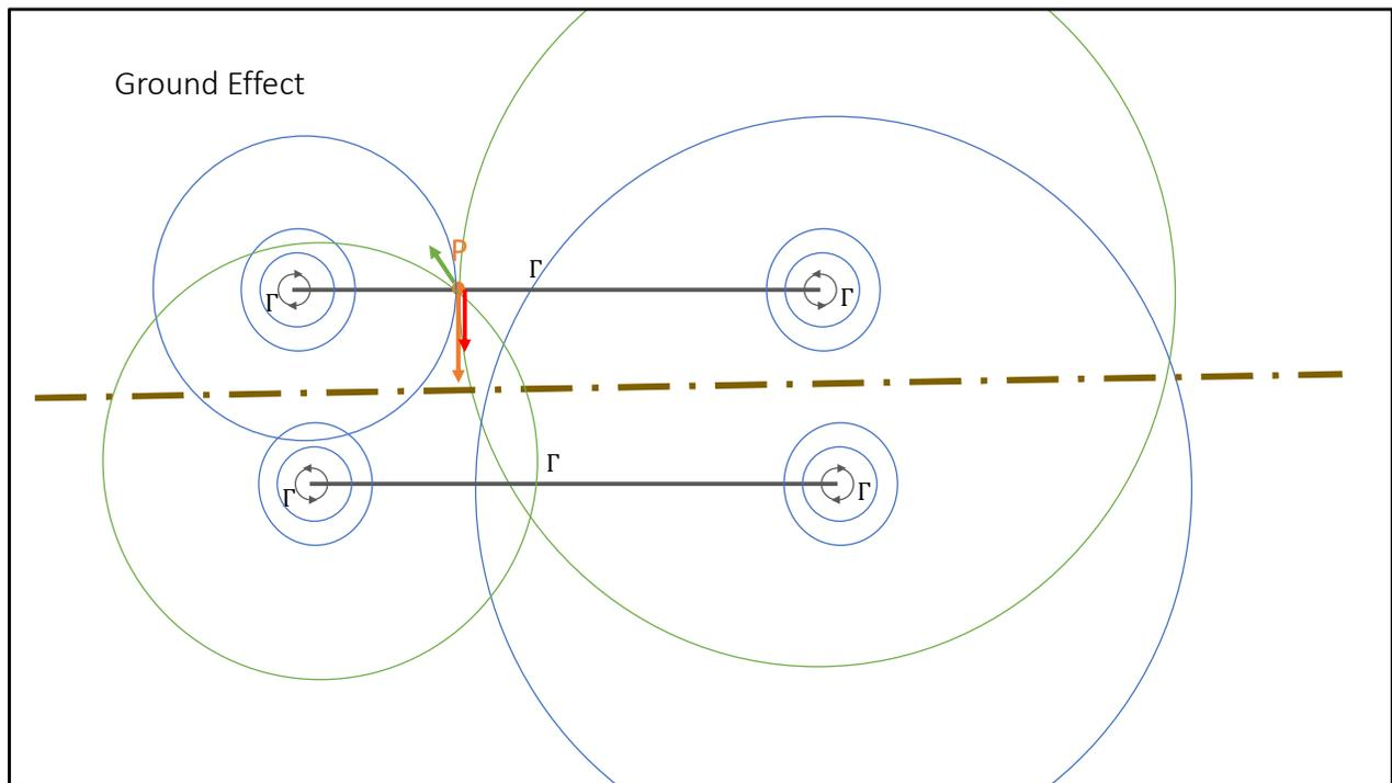
A useful trick is to place another “wing” (vortices system) symmetrically with respect to the ground plane, as shown above. By symmetry, no flow can penetrate the axis of symmetry, and the flow pattern in the upper half resulting from this configuration will thus be the same as the flow pattern in presence of the ground plane!
