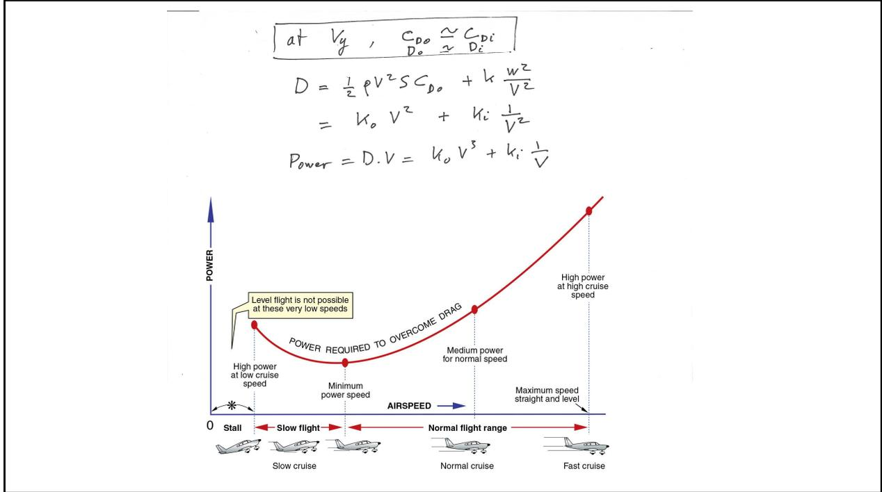
How does induced drag compare to parasite drag? A useful rule of thumb is that, at best rate of climb speed ( $V_y$ ), induced drag is approximately equal to parasite drag. At lower speeds, induced drag dominates, at higher speeds, parasite drag does.
