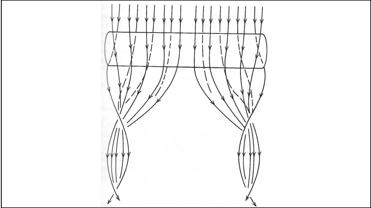
The flow around the wingtip displaces the streamlines towards the wingtip on the lower surface (dashed) and away from the wingtip on the upper surface (solid) . Combined with the freestream velocity, this spanwise flow creates a swirling motion downstream of the wing, resulting in two trailing vortices. Ley’s note that, while these vortices are commonly referred to as “wingtip vortices,” they origin spans the entire wingspan.
