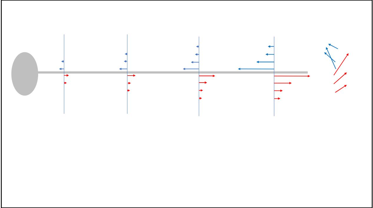
View from behind the trailing edge, looking forward (fuselage on the left, wingtip on the right). Red arrows show the spanwise flow (crossflow) on the lower surface, blue on the upper surface. A shear layer is present at the trailing edge.
